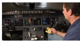
A Landmark Aviation technician downloads engine and systems data onto a disk for troubleshooting.
