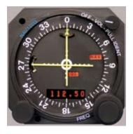
Narco's NAV 122D is a self-contained 200channel navigational receiver, 40-channel glideslope receiver, VOR, localizer and glideslope indicator.
