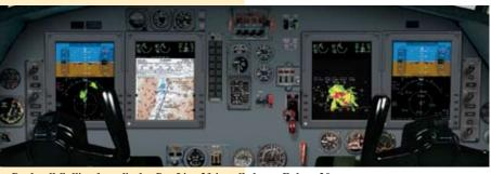
Rockwell Collins four-display Pro Line 21 installed on a Falcon 20.
