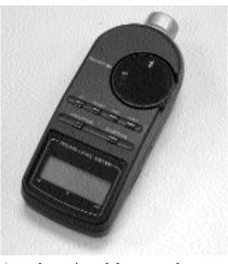
A sound meter is needed to accurately meas ure the ambient noise in cruise and to set the audio alerts.
