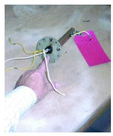
Defective potted feed-through on stand-off assembly.
