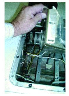
Autopilot servo is held out of the way to show fuel probe stand-off and wiring is in its native element.
