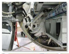
Premier Air Center/ West Star Aviation gives this Falcon 50 the four-tube EFI-890R installation, including Vision-1, Class A TAWS, dual UNS-1E FMS, P-880 radar, Collins AH-3000 AHRS, dual Universal radio control units, and dual Baker M-1035 audio nanels
