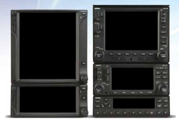
Garmin's new GTN 650/750 series (left) is smaller, with a bigger screen and touch-screen controls than the older, larger stack (right) with dials and knobs.
