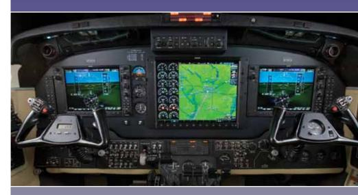
Elliott Aviation recently announced it will offer the Garmin G1000 Integrated Avionics Suite glass cockpit in a Beechcraft King Air 300/350. According to Elliott Aviation, the company has retrofitted more King Airs with the G1000 than all other dealers/installers combined.
