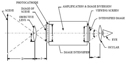
Figure C-1. Diagram of an image intensifier.
