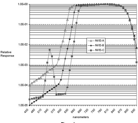
Figure 1. Relative spectral response characteristics of Classes A.B and C NVIS.
