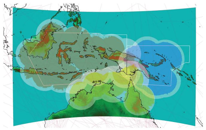
One of Australia's objectives in its region is to share ADS-B data between states to improve FIR (Flight Information Region) boundary safety. This approach is well accepted by the Asia pacific ICAO states. Note: This particular graphic does not include most Australian ADS-B ground stations and the plans in Indonesia and PNG are quite fluid.
